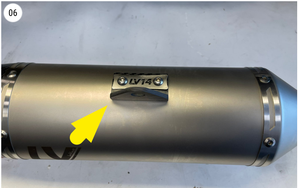
Fit the bracket on the muffler
